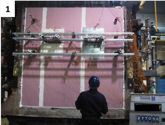
Flexible wall = Gypsum wall
