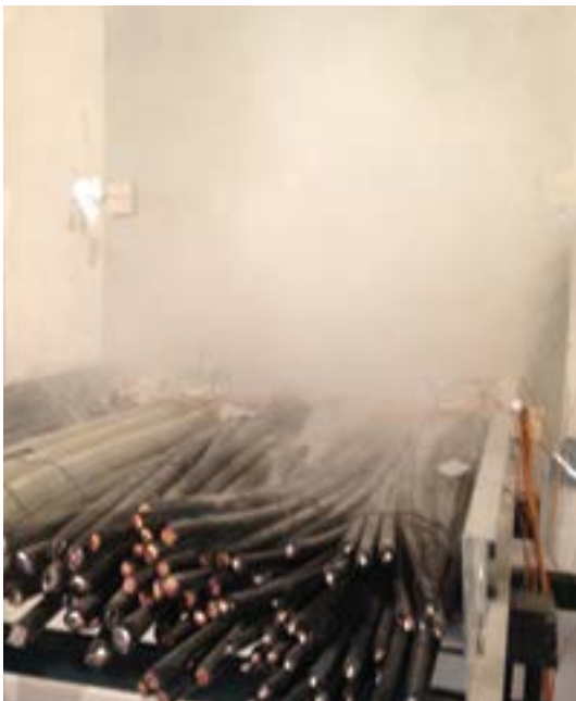
ILL 3. Horizontal Air Leakage Test. © 2020 UL LLC. Reprinted with permission.
