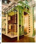
support Canadian industry, government and academia in basic fire-resistance research, technology development and testing. The complex contains a 3-story Burn Hall test facility, a full-size stair, elevator and service shaft, as well as a tunnel facility that can accommodate a full-size rail or subway car to perform almost full-scale testing not usually
