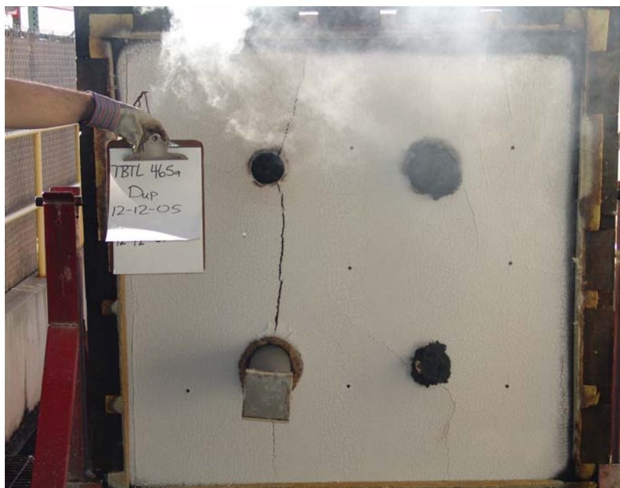
On Sept. 20, 2007 UL 1479 required that all penetrants be exposed to furnace conditions such as shown here
