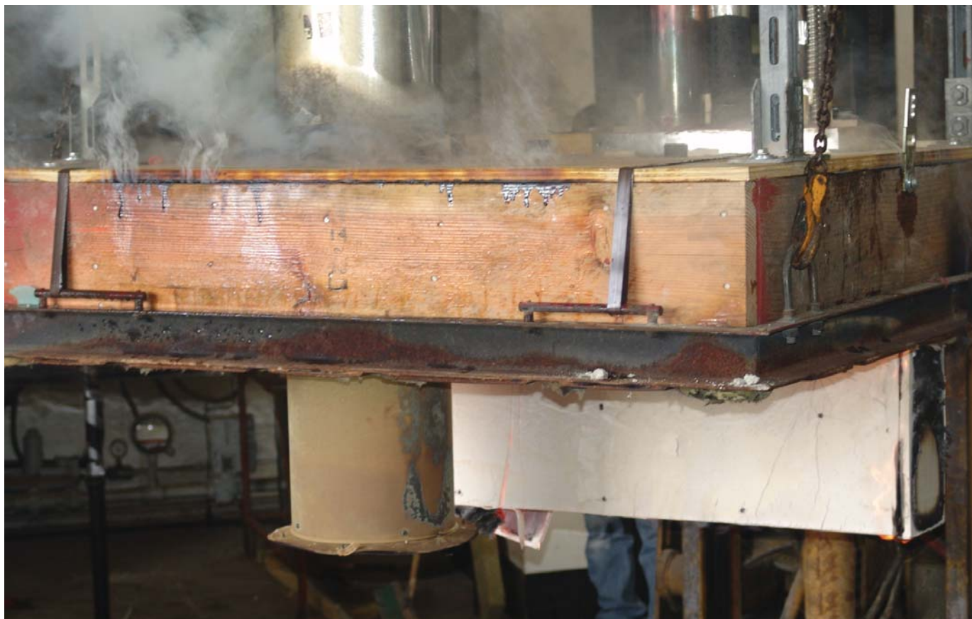
Penetrant on left is not contained within chase wall. Penetrants on right hand side are contained within a chase wall.
