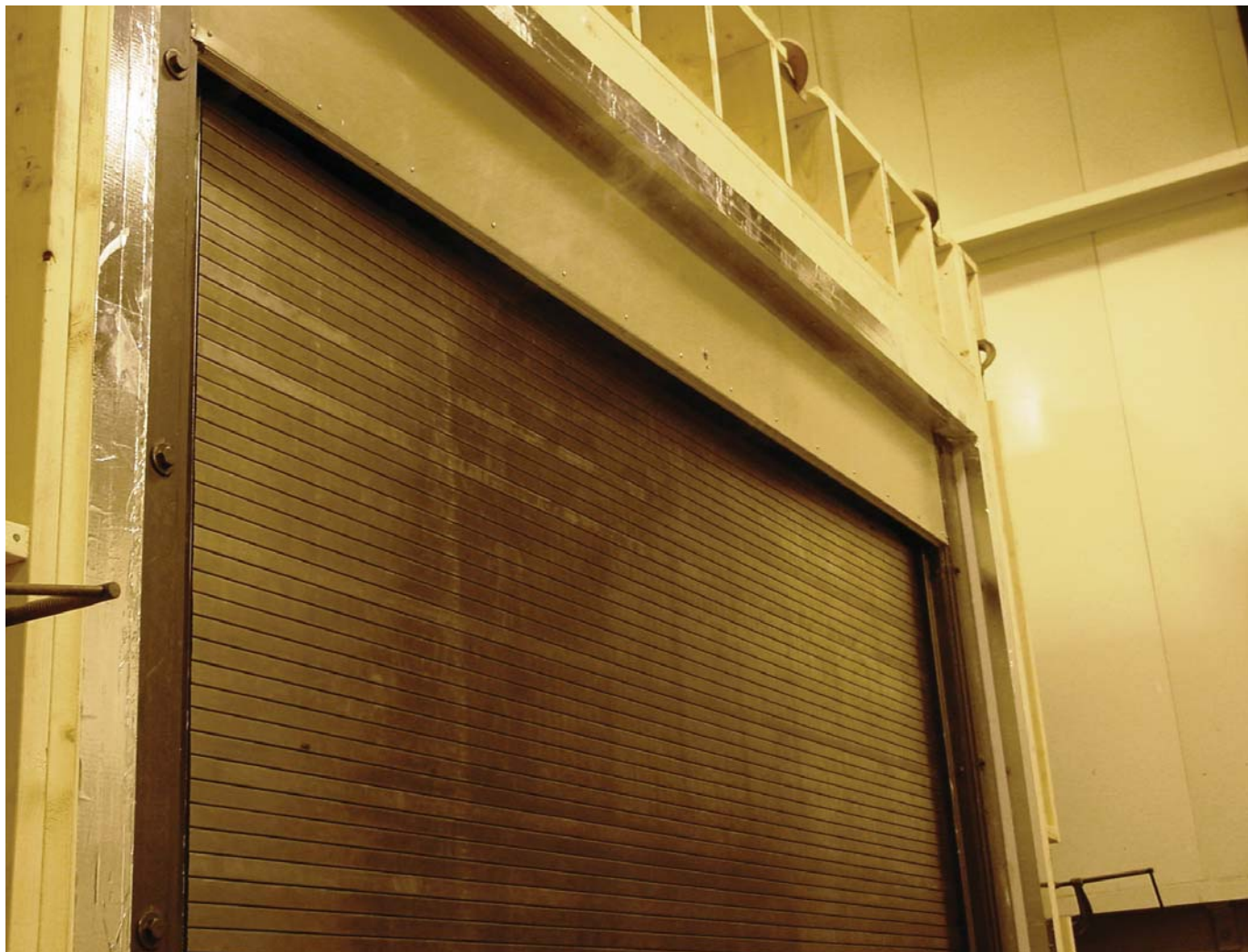
Rolling fire door being subjected to UL 1784 Air Leakage Tests
