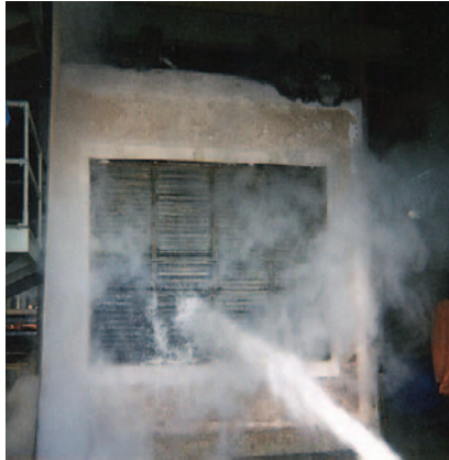
Combination Fire/Smoke Damper during Hose Stream Test. Nailor Photo.
