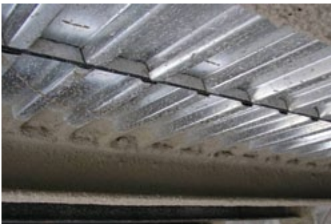
Fire-Resistance Rated Assembly, Large Scale Furnace. UL Photo.
