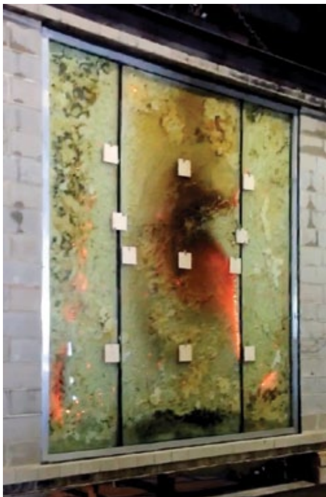
Radiant Heat Test. SAFTI FIRST photo.
