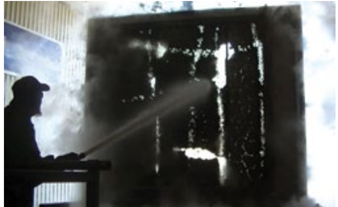
Hose Stream Test. SAFTI FIRST photo.
