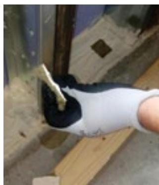
Cuts in the profile of firestop spray products reveals assembly thickness. Firestop Southwest Photo.
