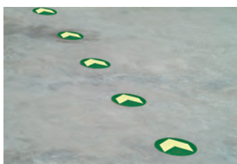
Enamel round markings with a pin (drill hole into concrete floor; fill in construction adhesive; insert pin into hole and place enamel flush on floor).
