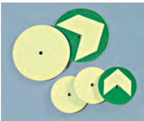
Enamel round markings with a pin (drill hole into concrete floor; fill in construction adhesive; insert pin into hole and place enamel flush on floor).
