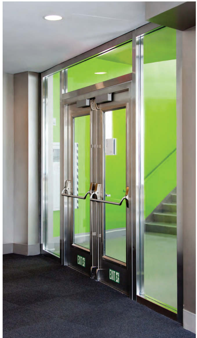
For this 2-hour stairwell, SuperLite II-XL 90 is used to exceed 100 sq. in. in the door vision panels while SuperLite II-XL 120 in Stainless Steel GPX Framing is used for the sidelites and transoms. SAFTIFIRST Photo
