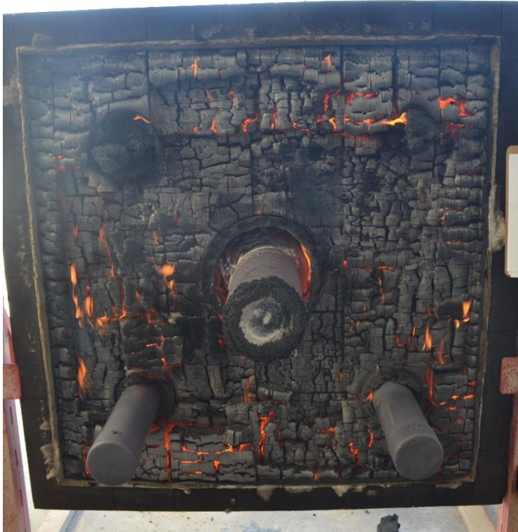
Fig. 13: CLT1 Exposed Side, Post Fire Endurance (Ref. 5)
