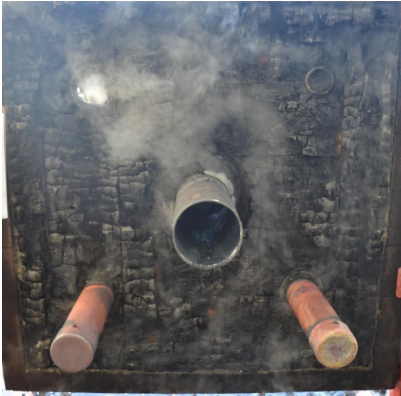
Fig. 16: CLT 1 Exposed Side Post Hose Stream (Ref. 5)
