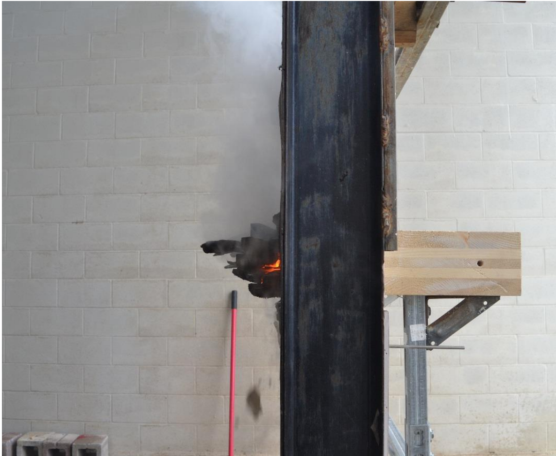
Fig. 20: Test Assembly Profile, Post Fire Endurance (Ref. 5)
