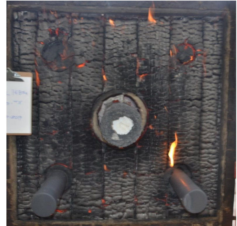
Fig. 15: CLT3 Exposed Side, Post Fire Endurance (Ref. 5)
