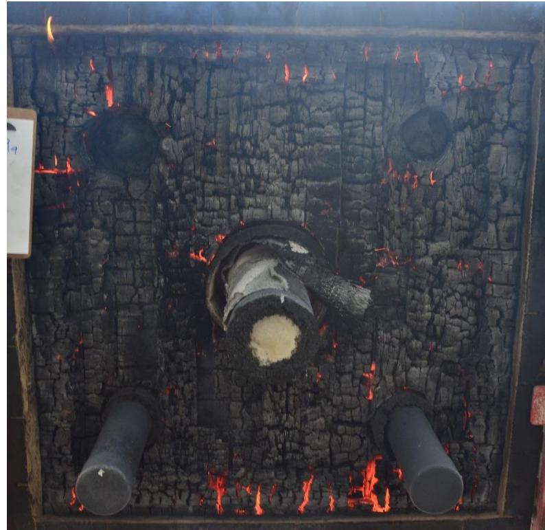
Fig. 14: CLT2 Exposed Side, Post Fire Endurance (Ref. 5)
