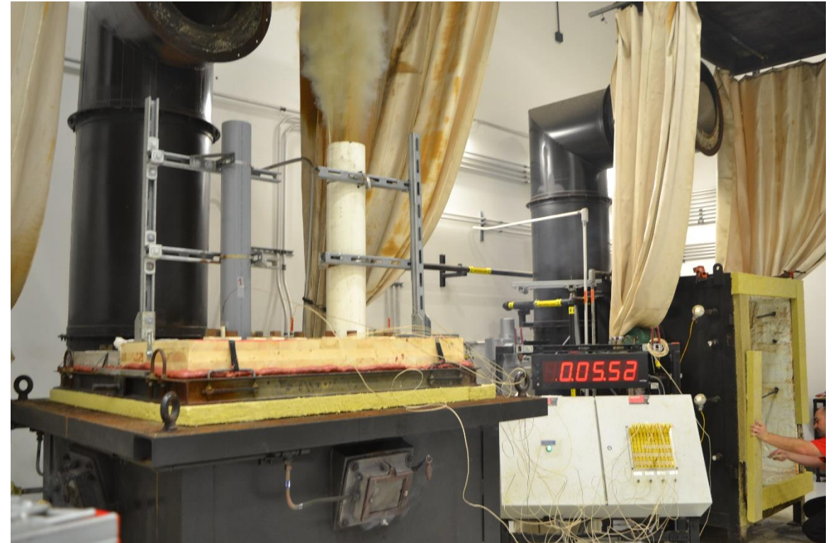
Figure 21: Nonexposed side of a CLT test assembly during a CAN/ULC S115 penetration test at 50Pa. Photo courtesy of Hilti Inc.
