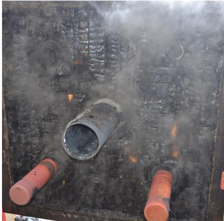
Fig. 17: CLT2 Exposed Side, Post Hose Stream (Ref. 5)
