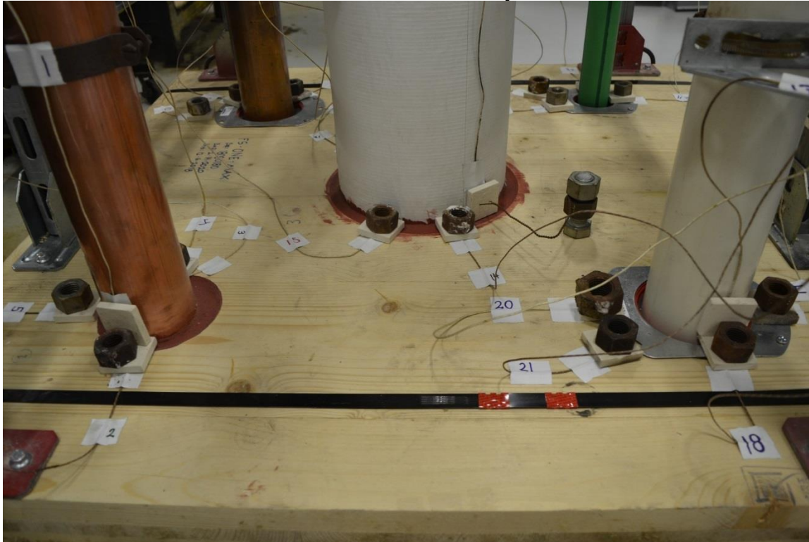
Fig. 10: CLT 1 Non-Exposed Side, Pre-Fire Endurance (Ref. 5)
