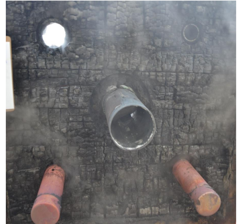
Fig. 18: CLT3 Exposed Side, Post Hose Stream (Ref. 5)
