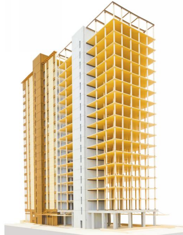
Figure 3: Rendering of Brock Commons Structural Frame (Ref. 2)
