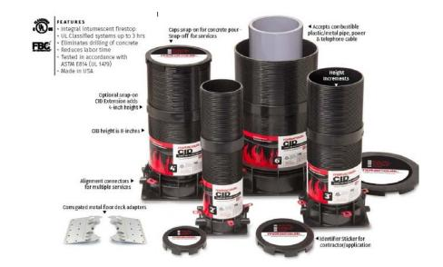
Cast In Devices are an all-in-one through penetration firestop devices that are installed before concrete pouring instead of post pour core drilling and firestopping.
