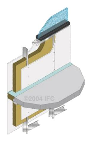
Along with sealing the slot area, a well engineered system provides structural protection and maximizes the integrity of the wall system...
