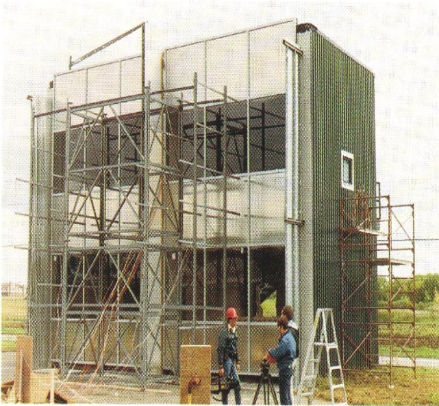
Fig. 1. Face of full-scale, permanent, fire-test facility at USG Corporation Research Center is set up for curtain wall fire test. Metal frame supports thermocouples for measuring flame plume temperature. Left side is "THERMAFIBER Curtain Wall Insulation Unit"; right side is "Glass Fiber Unit."
