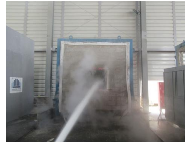
Picture 15: The specimen during the hose stream test.
