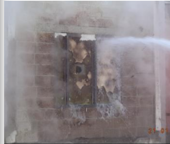
Picture 7 – During the Hose Stream Test the seal had come off allowed the passage of water to penetrate to the unexposed face @ 0
