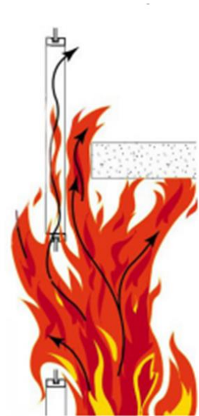
Unprotected Perimeter Joint
