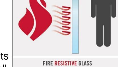
When use in walls, both glass and frame must block passage of heat
