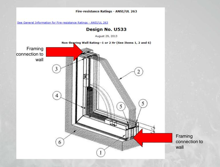
Steel Framing Members\* — Nom 4-1/4 in. (2 hr /TGP 120) and 3-1/2 in. (1hr /TGP 60) wide with lengths cut according to glazing opening size. Secured to steel studs with No. 10, 4 in. long self drilling, self tapping buglehead screws spaced nominally 18 in. OC.
