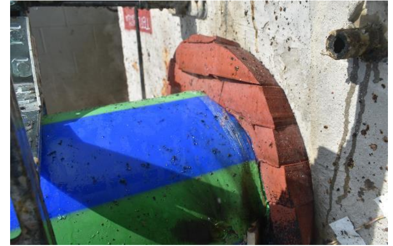
Nonexposed side, post fire endurance
