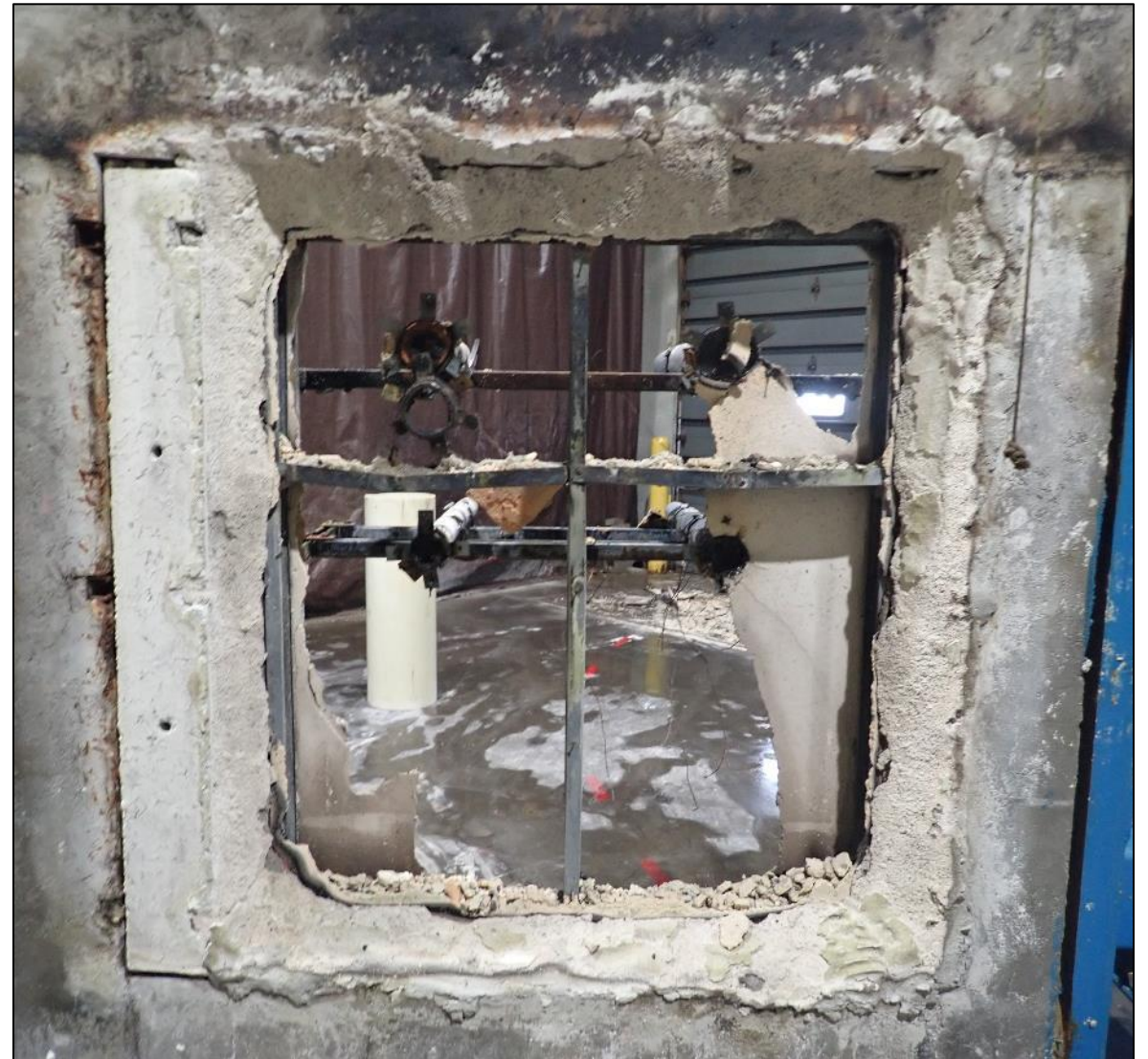
Hose Stream Test after 2 Hours 38 Seconds @ 30 PSI
