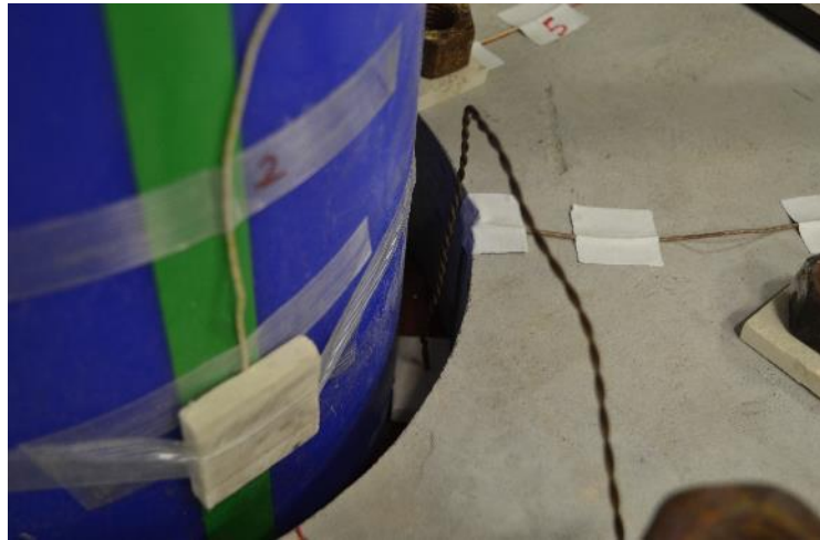
Nonexposed side, before fire endurance
