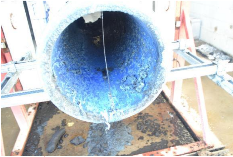
Nonexposed side, post fire endurance, showing pipe left open/vented
