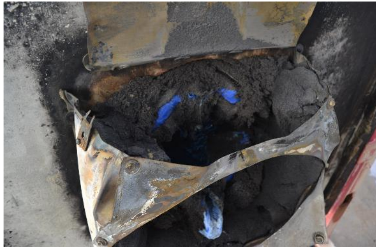
Exposed side, post fire endurance (46 minutes). Damage to steel enclosure from expanding intumescent
