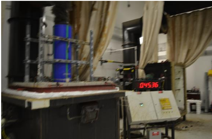
Nonexposed side, pipe vented at 45 minutes
