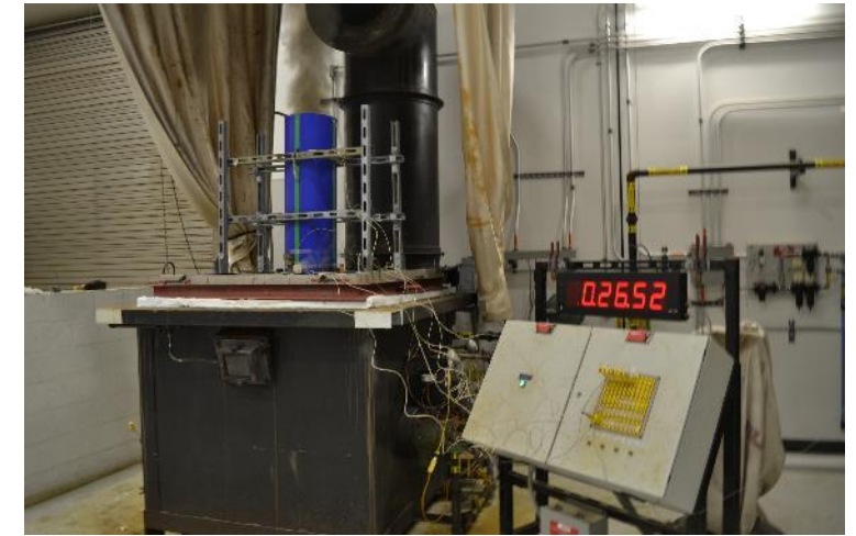
Nonexposed side, fire endurance, pipe has not fully vented
