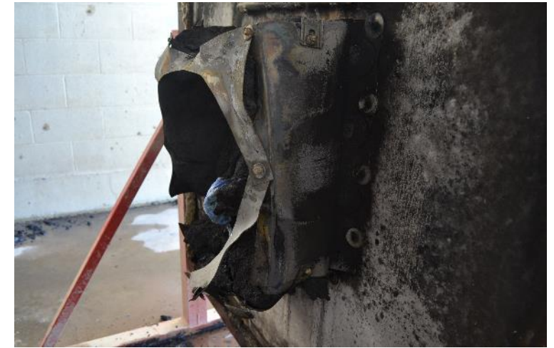
Exposed side, post fire endurance (46 minutes). Damage to steel enclosure from expanding intumescent
