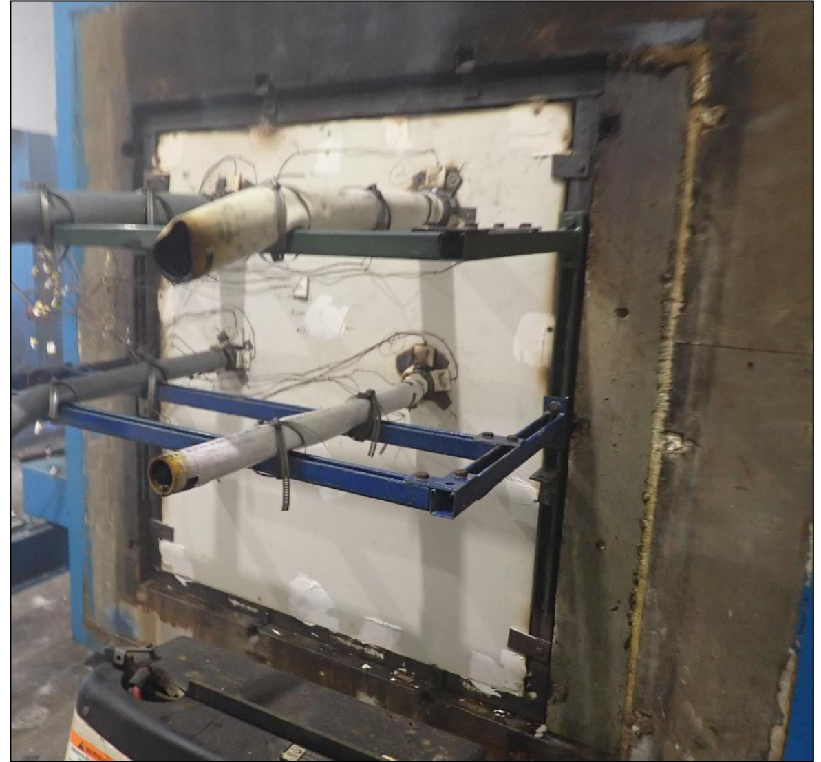
Pipes on Unexposed Side After 2 hours
