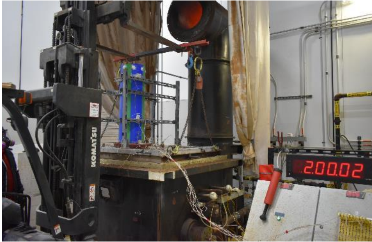
Nonexposed side, end of fire endurance
