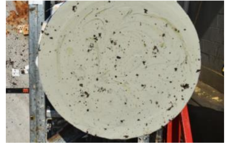
Nonexposed side, post hose stream
