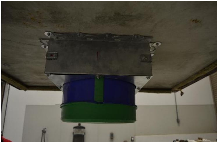
Exposed side, before fire endurance. Pipe capped on exposed side. Solution same as cUL C-AJ-2836, wrap strip housed in metal enclosure.
