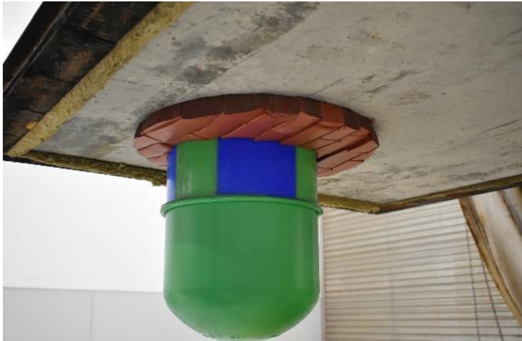
Exposed side view before fire endurance. Shows pipe closed on exposed side. Firestop block solution.
