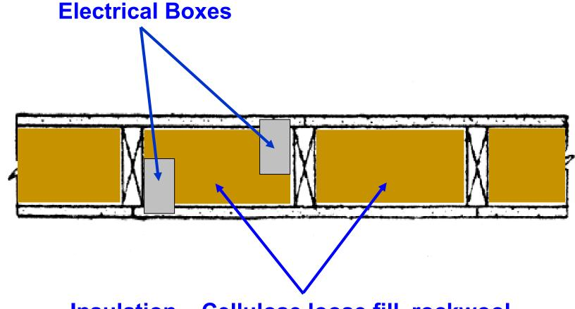
Insulation – Cellulose loose fill, rockwool or slag mineral wool
